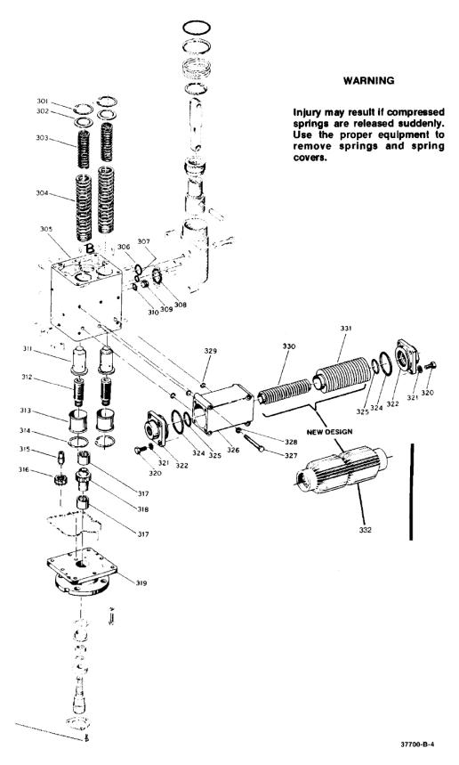
Figure 6-4. Power Case and Oil Cooler, EGB-35P/-50P
