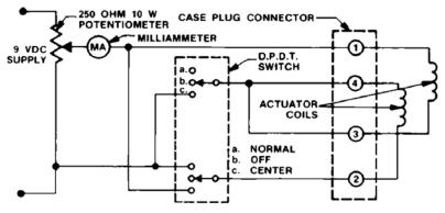
Figure 3-1. EGB Electrical Test Circuit
