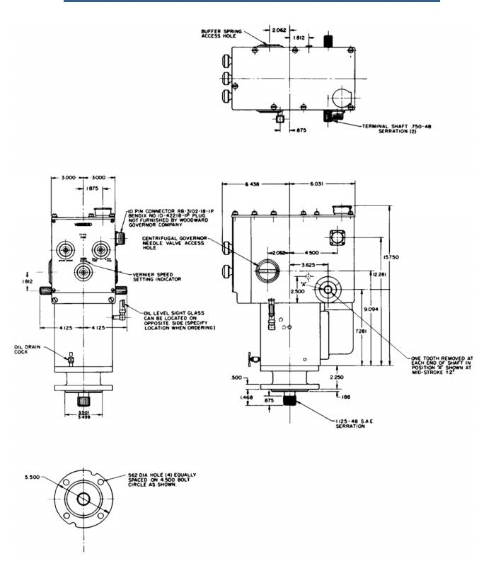
Figure 2-2. EGB-10P and 13P Exterior Dimensions
