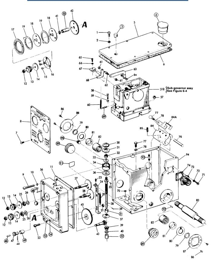
Figure 6-1. Column Assembly Parts, EGB-10P/-13P/-35P/-50P
