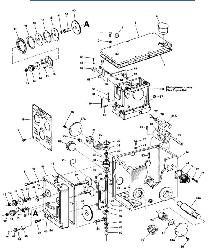
Figure 6-9. Column Assembly Parts, EGB-29P/-58P
