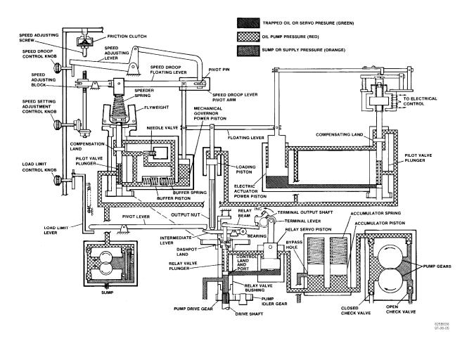
Figure 4-1a. EGB-10P and 13P Schematic
