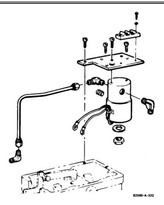
Figure 1-3. EGB Shutdown Solenoid
