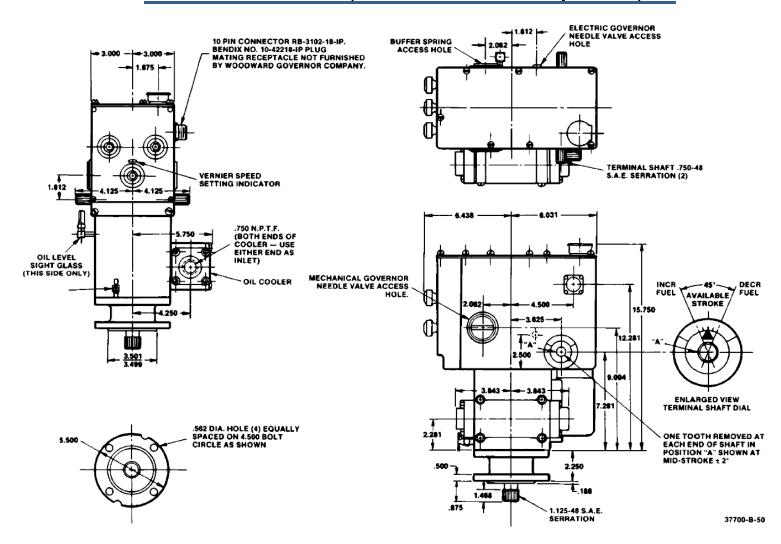
Figure 2-3. EGB-35P and 50P Exterior Dimensions
