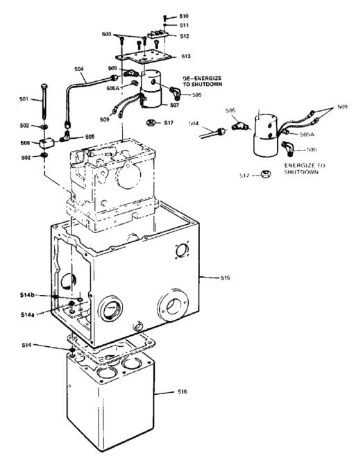
Figure 6-6. Solenoid Shutdown (optional)
