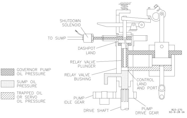
Figure 4-2. Schematic View of Relay Valve Plunger with Shutdown Solenoid (see Shutdown Solenoid explanation in Chapter 1)
