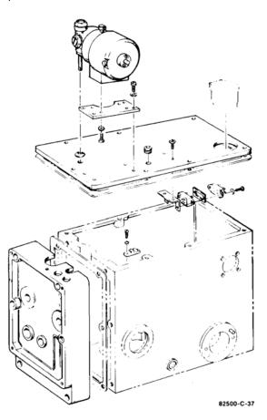
Figure 1-2. EGB Speed Setting Motor
