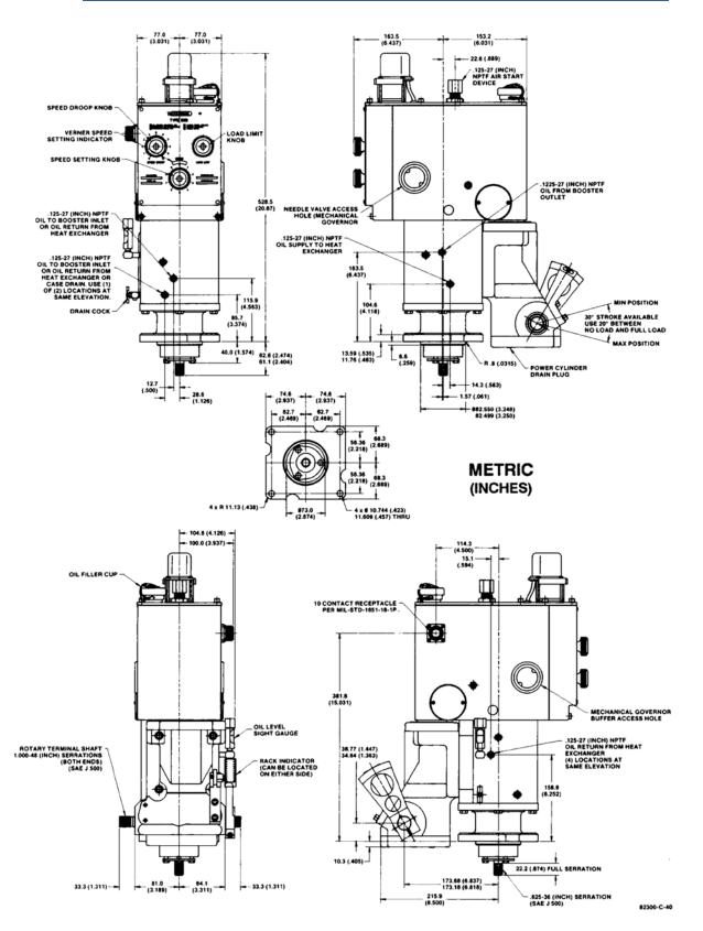
Figure 2-5. EGB-29P and 58P Exterior Dimensions
