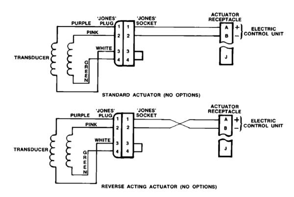
Figure 5-1. Typical Schematic Wiring Diagram of Governor/Actuator
