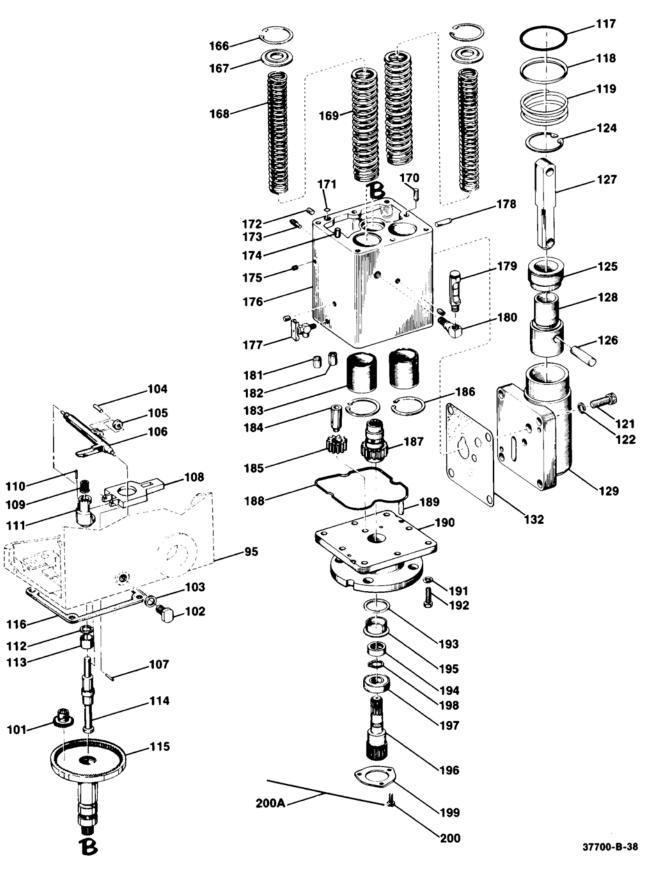
Figure 6-2. Power Case and Power Piston, EGB-10P/-13P
