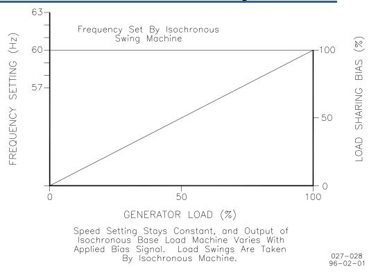
Figure 5-9. Isochronous Base Load on an Isolated Bus
