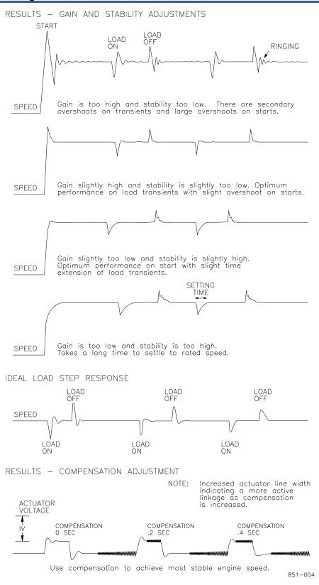
Figure 3-4. Typical Transient Response Curves
