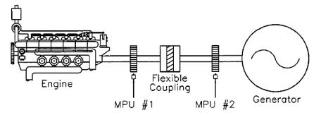
Figure 1-1. Flexible Coupled Generator Set
