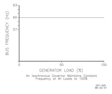
Figure 5-6. Isochronous Mode
