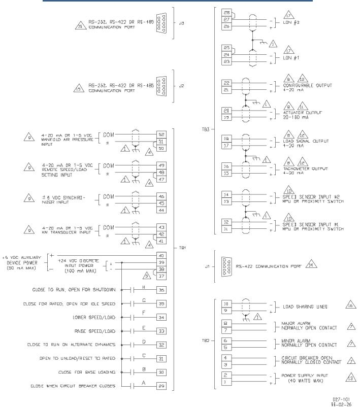
Figure 1-5. Plant Wiring Diagram
