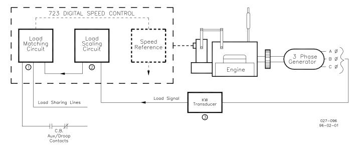
Figure 5-4. Paralleling System
