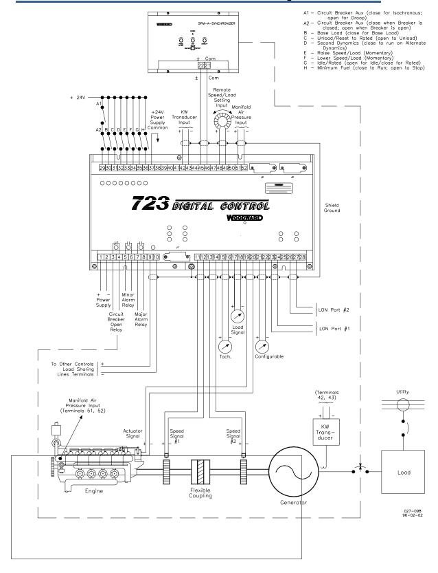
Figure 1-4. Typical 723 Connections
