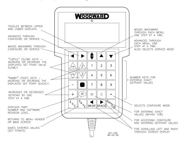
Figure 3-1. Hand Held Programmer Functions
