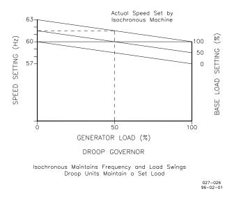
Figure 5-7. Droop/Isochronous Load Sharing
