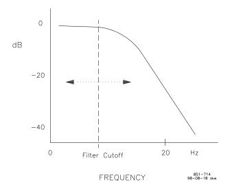
Figure 3-5. Speed Filter
