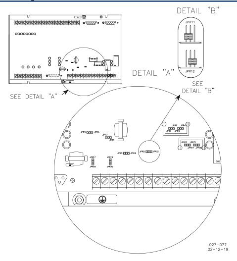
Figure 2-1. 723 Control Internal Jumpers
