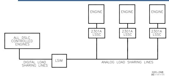
Figure 4-2. How the Analog Controls See the LSIM (all of the DSLC-controlled engines appear as a single load sharing unit)
