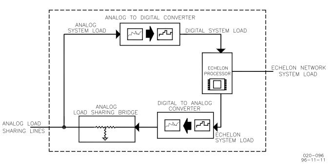
Figure 4-3. Block Diagram of the LSIM
