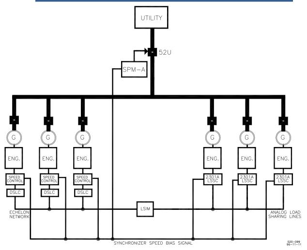
Figure 4-4. Example of Possible Existing Synchronization Method Using the SPM Inputs to the 2301A LSSCs
