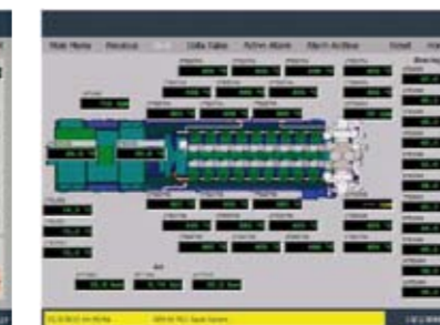
All values at a glance: Genset values are logged for diagnostic and proactive maintenance.
