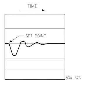
Figure 13-8. Typical Response to Load Change
