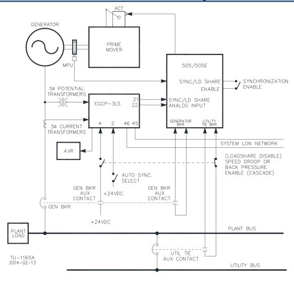
Figure 9-15. EGCP-3 LS Interface Wiring
