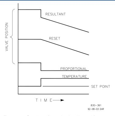
Figure 13-2. Open Loop Proportional and Integral Response
