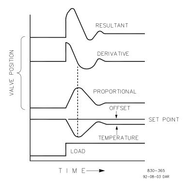
Figure 13-5. Closed Loop Proportional and Derivative Action
