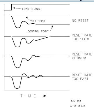
Figure 13-4. Integral Gain (Reset) Setting Responses
