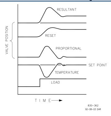
Figure 13-3. Closed Loop Proportional and Integral Response
