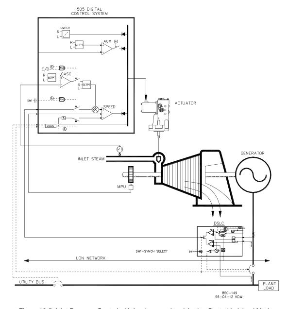
Figure 10-5. Inlet Pressure Control with Isochronous Loadsharing Control in Island Mode
