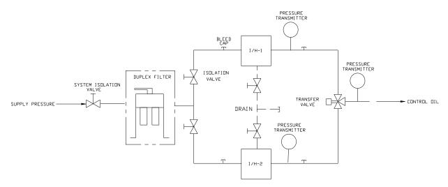
Figure 9-16. Typical Redundant I/H System with a Transfer Valve
