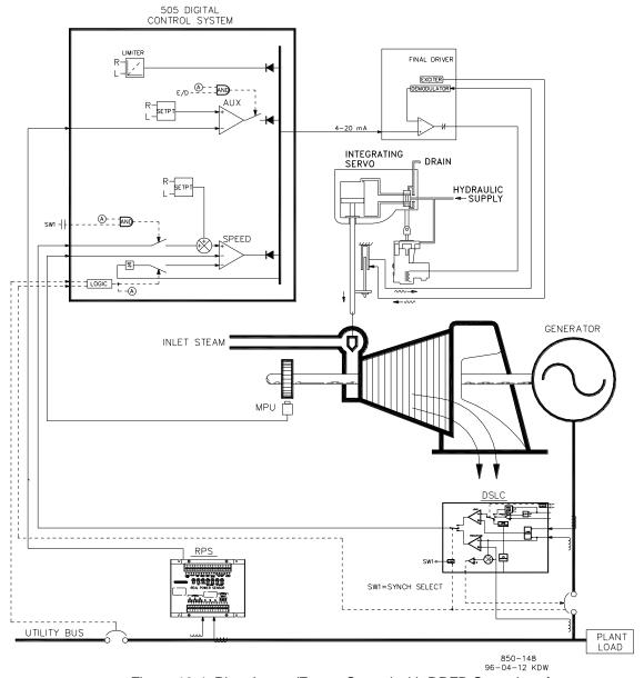
Figure 10-4. Plant Import/Export Control with DRFD Servo Interface
