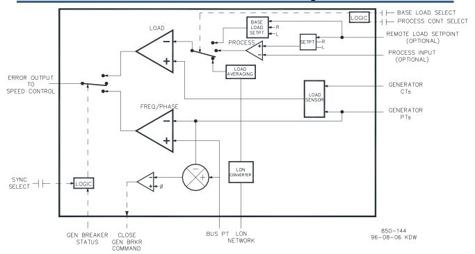
Figure 9-14. EGCP-3 LS Functional Diagram
